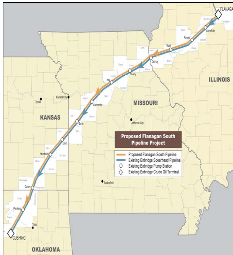
Figure 4. Proposed Enbridge Flanagan South Pipeline Route
