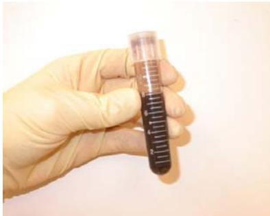
Fig. 6. A vial of liquid sample from an APDS system, showing the heavy background contamination and sample complexity encountered in field biodetection missions.
