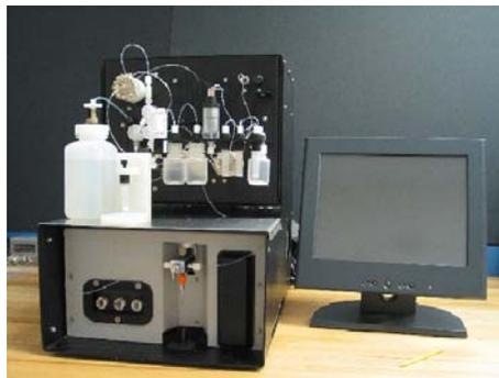
Fig. 5. The compact FluIDx unit is a point-of-care multiplex medical diagnostics system that uses the automated fluidics and bead-based immunoassay platform of the APDS. It has been used to rapidly diagnose viral upper respiratory infections.
