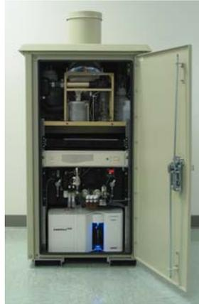
Fig. 2. The Autonomous Pathogen Detection System (APDS) is a self-contained biodetection system with automated sample collection, computer-controlled fluidics, wireless communications, and two independent types of bioassays.
