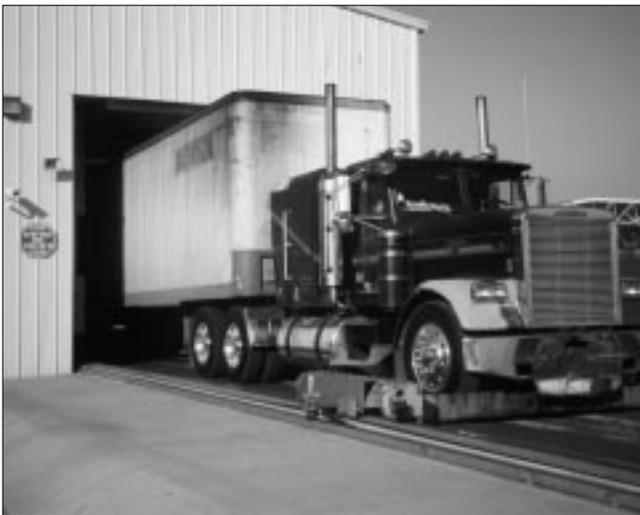
Truck X-ray facility, Otay Mesa, CA, used principally by U.S. Customs for drug interdiction. A detailed X-ray of an entire semi-truck with cargo requires 10 minutes.
