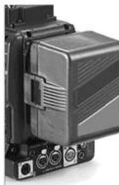
Extended-life 160 watt-hour lithium ion battery.
