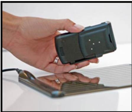
**Power pad:** Delaware-based WildCharge has developed an electrically conducting pad that charges phones and other devices via adaptors. Above, the battery cover of a Motorola Razzr mobile phone has been replaced by WildCharge's adaptor, which has four metal contacts arranged in a Y shape. *Credit: WildCharge*
