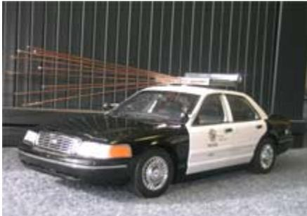
**Zapping the bad guys:** Attached to the roof of this police car is a 200-pound electromagnetic system that can quickly bring an opposing vehicle to a stop. The system is six to eight feet long (antennae included) and almost three feet wide. It works by sending out pulses of microwave radiation that disable the microprocessors that control the central engine functions of a car. **Credit: Eureka Aerospace**
