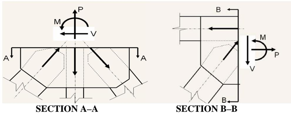
Figure 2. Gusset Plate Design Sections.
