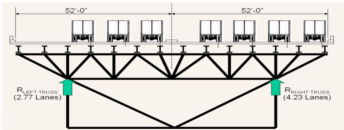
Figure 1. Live Load Lane Placement Used for Design.
