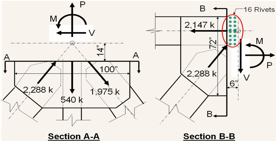
Figure 4. Gusset Plate U10 Free Body Diagrams.
