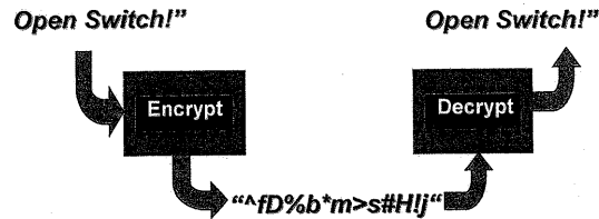
Figure 2 – AGA 12 specifies that the messages (Open Switch here) are encrypted inside a secure facility so that they are “scrambled” and can not be read. They are thus unreadable while they are on the insecure network, but can be decrypted and read properly when they are delivered to the second secure site.
