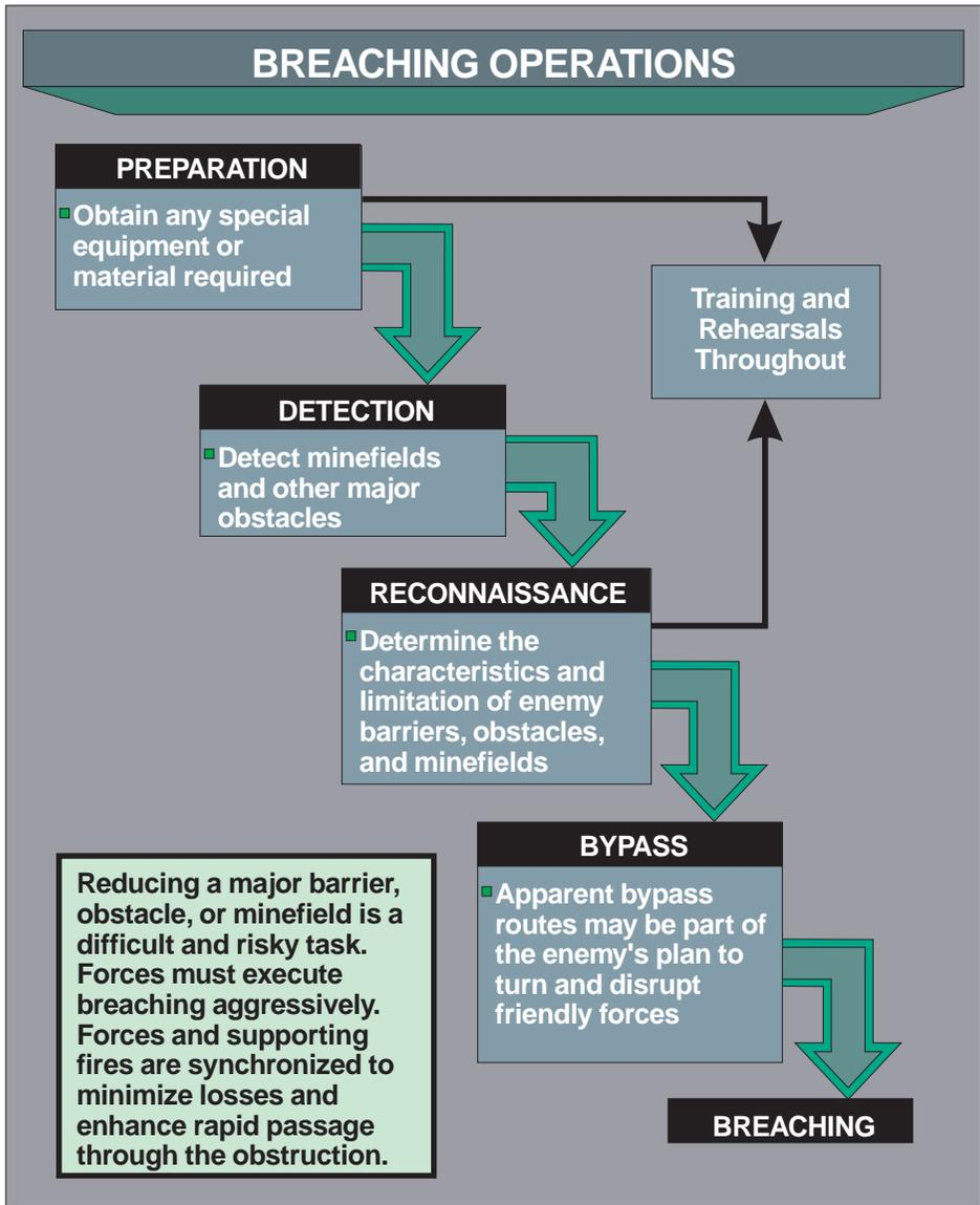
Figure IV-2. Breaching Operations
