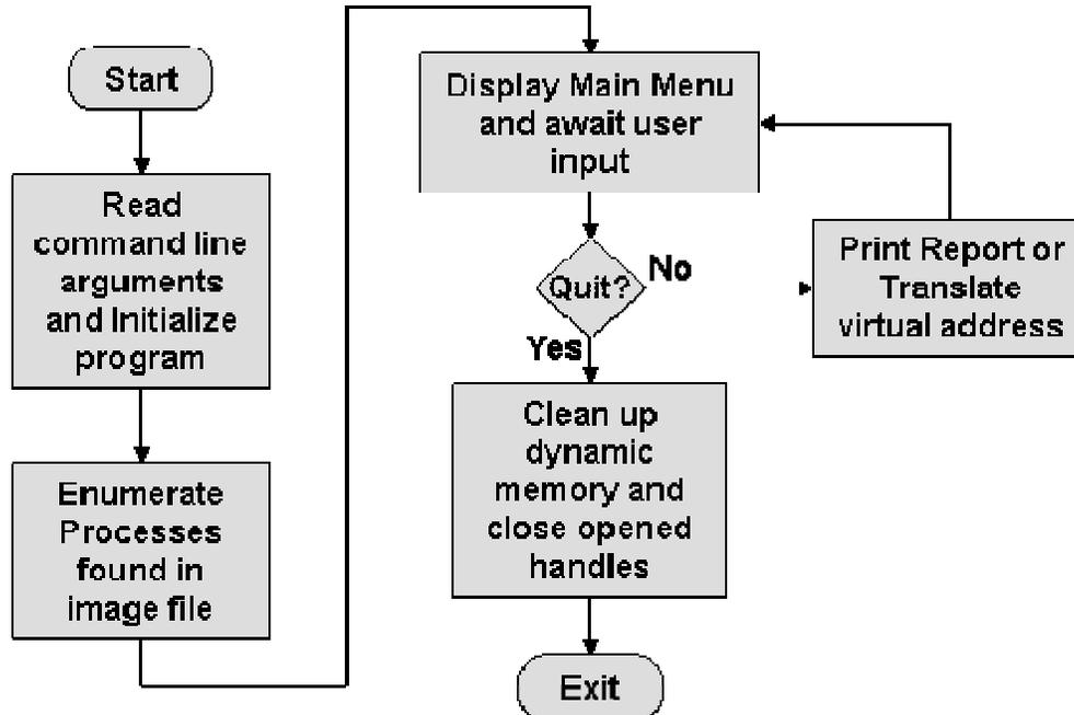
Figure 8 shows the general flow of the program, which is described in words below. The program uses the user command line inputs to initialize the program global variables setting the start address of the active process list and the page size for the
