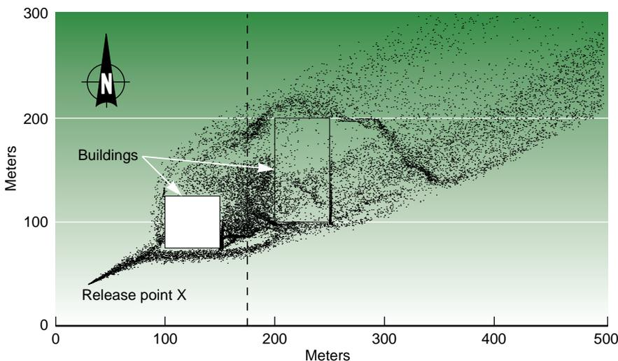
**Figure 4.** This scenario shows where particles will be 10 minutes after they are released at point X in a 240-degree (west southwest) wind of 10 meters per second. Several areas of high particle concentration are visible to the south of the two buildings, with lesser concentrations to the north and to the east.
