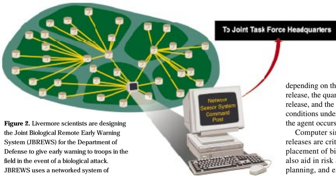
**Figure 2.** Livermore scientists are designing the Joint Biological Remote Early Warning System (JBREWS) for the Department of Defense to give early warning to troops in the field in the event of a biological attack. JBREWS uses a networked system of sensors that automatically report to a central computerized command post.
