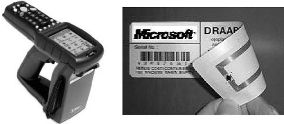
**Figure 8. Hand-held Scanner and Passive RFID Tag (PSC, 2006; Microsoft, 2006)**
