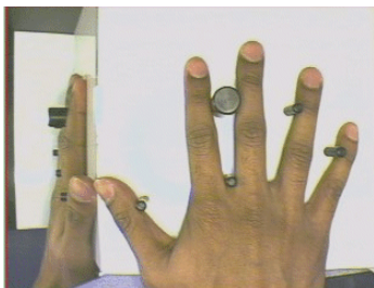
Figure 3: Hand Including Mirror Image as Seen by the CCD Camera. 5
