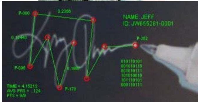
Figure 1: Dynamic Signature Depiction: As an individual signs the contact sensitive tablet, various measurements are observed and processed for comparison.<sup>1,2</sup>
