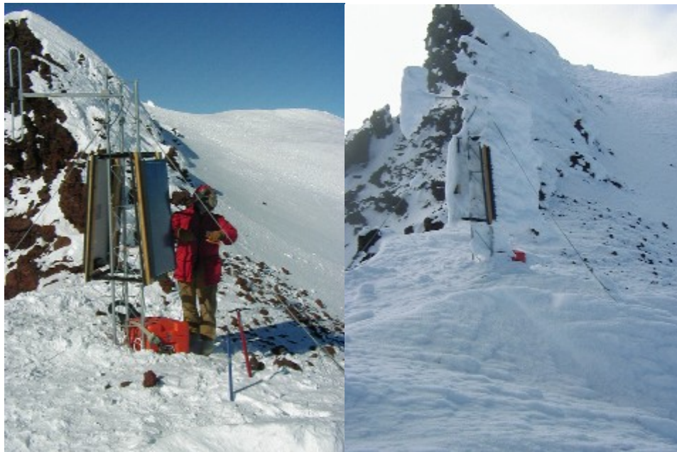
Figure 2.3. Two pictures showing the same repeater site on the top of Mt. Terror. The snow covering the repeater in the left picture is actually very hard and requires nothing less than an ice axe for removal.
