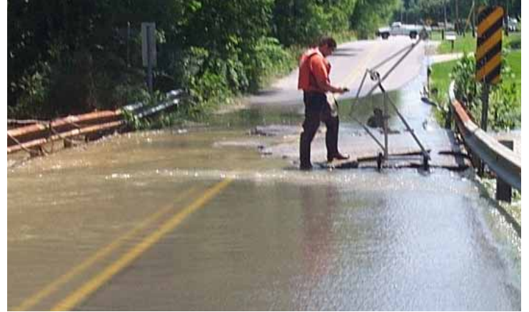
Kokomo Creek flows over the bridge in the town of Kokomo, Indiana, as a U.S. Geological Survey streamgager prepares to make a discharge measurement.
