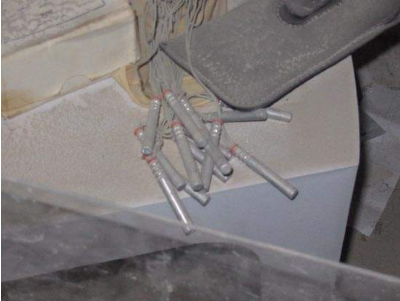
Blasting caps found in the chemical/explosives weapons laboratory in Fallujah. Official USMC Photo (Released)
