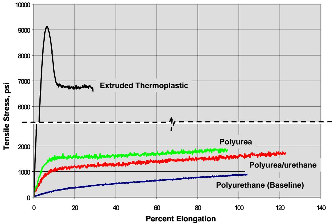
**Figure 5. Typical Results from Polymer Tensile Testing**
