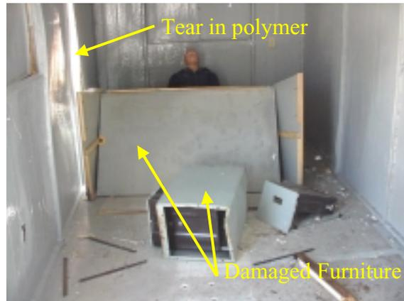
**Figure 11. Post-Test Interior View of Structure 1**
