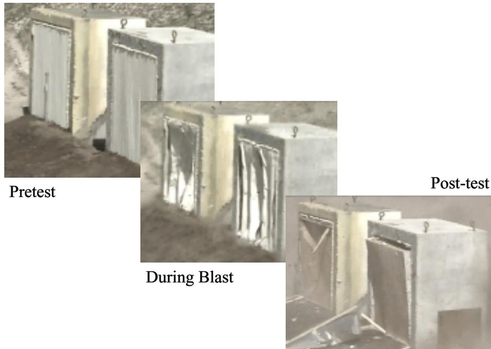
**Figure 7. Component Wall Test**
