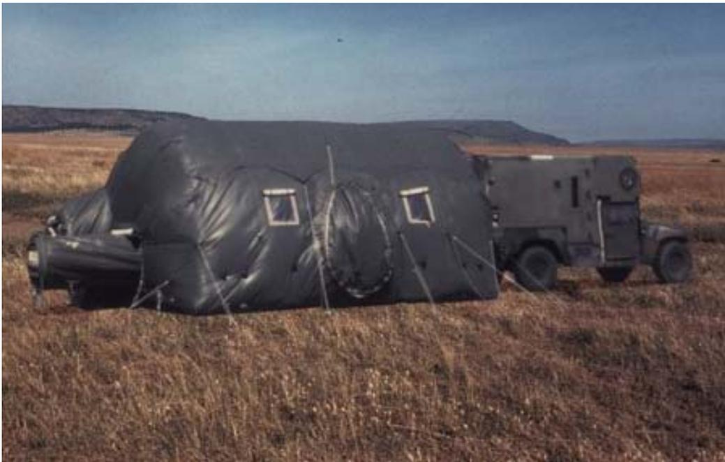
Figure 3. Chemically and biologically protective shelter system (CBPSS) of CHALLENGE® X-22 barrier laminate.
