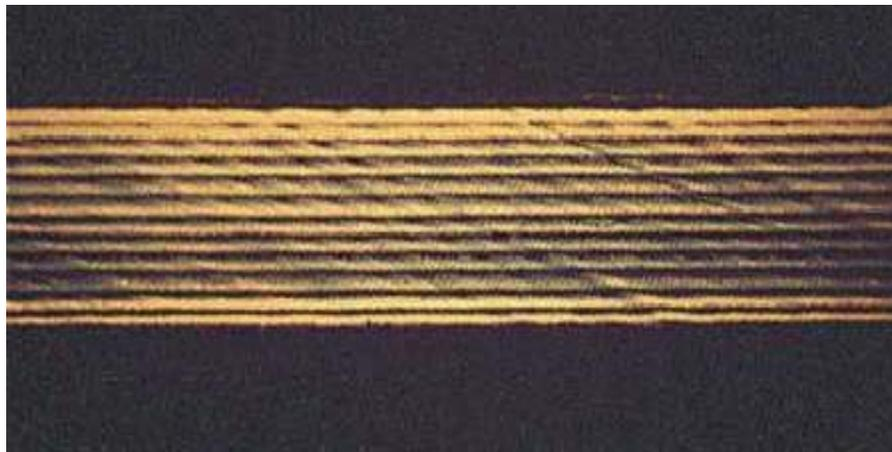
Figure 5. Cross-sectional photomicrograph of SGPPL cast PTFE film, 4 mils, 12 layers.
