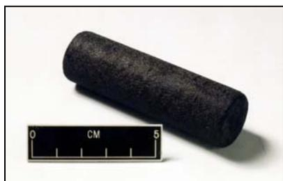
Figure 1. Carbon-bonded carbon fibre composite.
