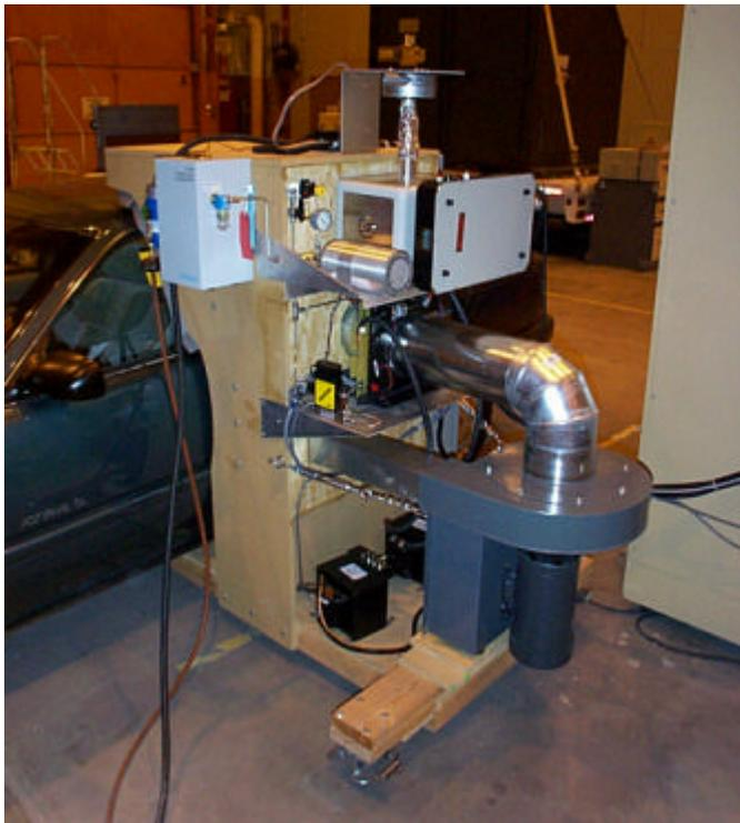
**Figure 4.** Prototype module for screening vehicles for explosives.
