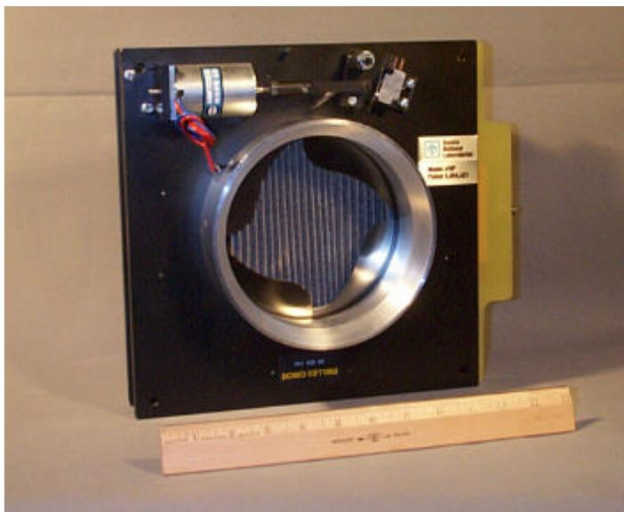
**Figure1.** The Sandia screen preconcentrator. Sampled air enters through the large round opening, and explosives molecules/particles are adsorbed on the pleated screen.
