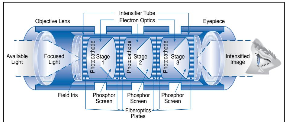
The tube is actually a sequence of three image intensifiers, each comprising a photocathode and phosphor screen.
