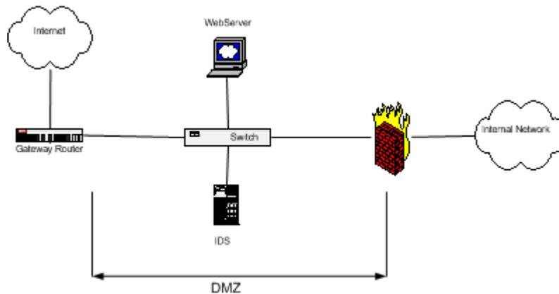
Figure 7. Illustration of DID with DMZ.
