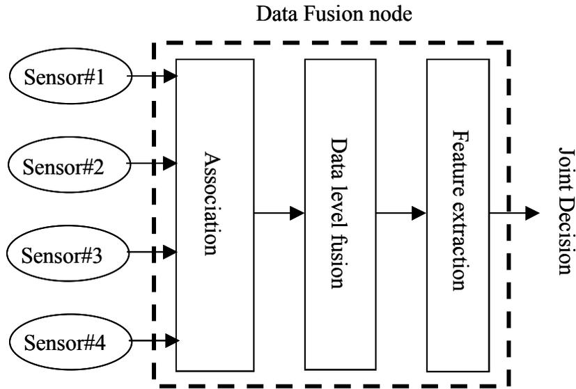
Figure 21. Direct level fusion (After Ref 11, pg. 1-7)
