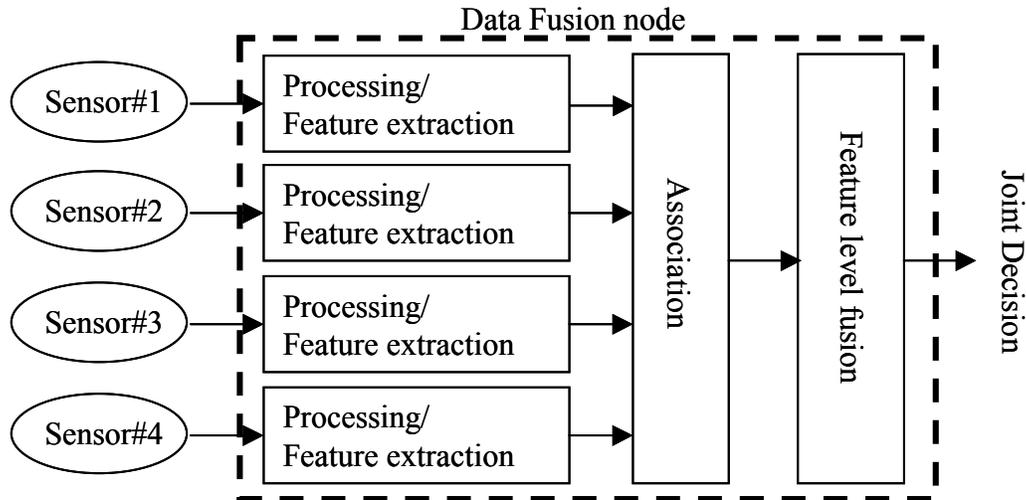
Figure 22. Feature level fusion (After Ref 11, pg. 1-7)
