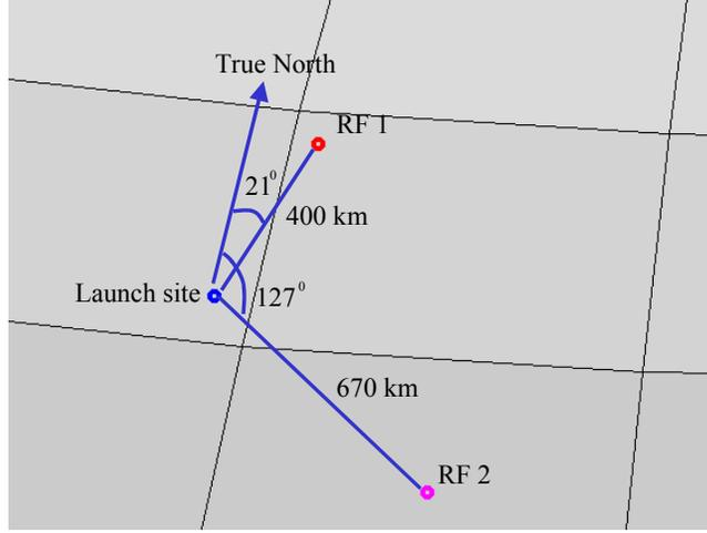
Figure 15. Locations of launch site and radar sensors
