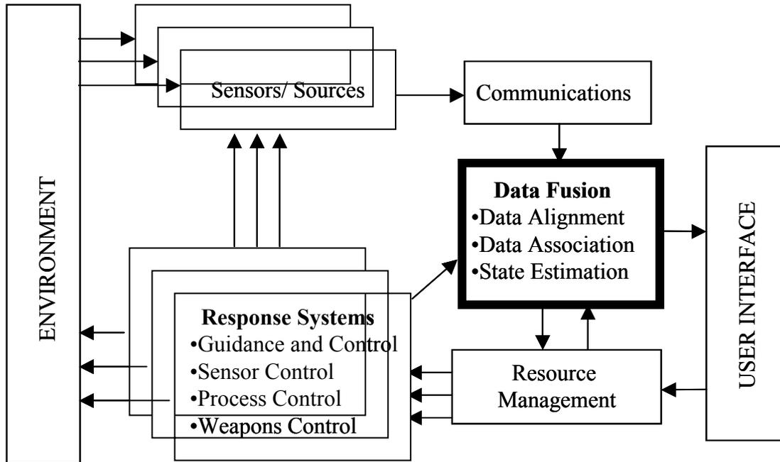
Figure 20. JDL Data Fusion Model (After Ref, 11 pg. 16-18)
