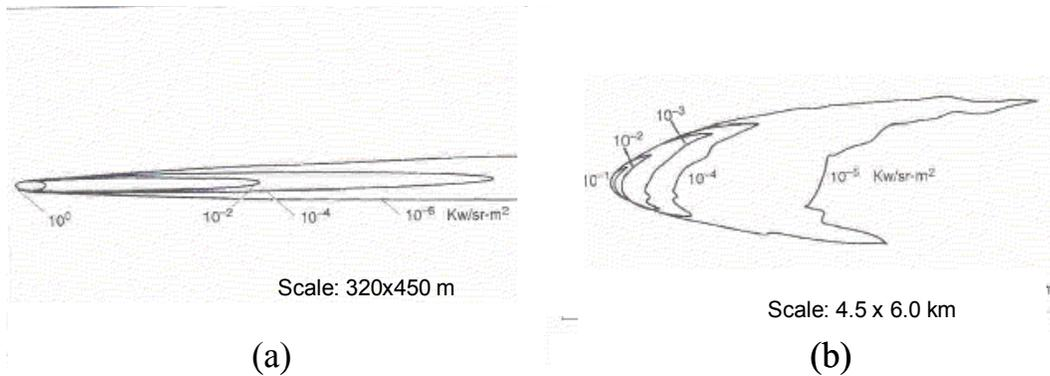
Figure 5. Radiance map of Titan IIIB for MWIR at altitudes 18 km (a) and 118 km (b) (From Ref 5)
