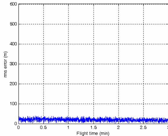
Figure 36. The rms position error using Bayesian technique.
