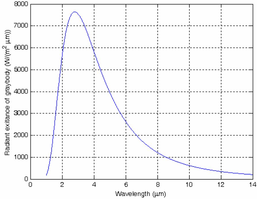
Figure 2. Radiant exitance of Titan IIIB (1035 K)
