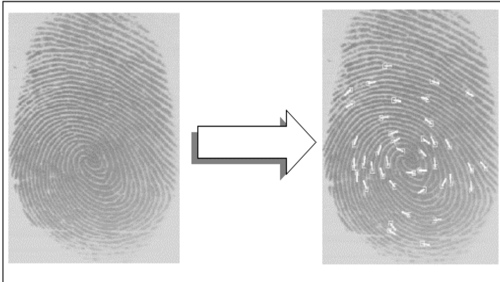
Figure 5. Finger Minutiae-Based Biometric Matching
