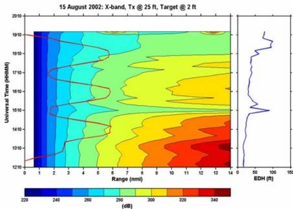
**Figure 1:** X-band 2-way loss out to 14 nmi as versus time-of-day. Right hand panel is calculated evaporation duct height. Estimated from lower atmosphere and ocean surface measurements and propagation model. Coastal region off Dam Neck, VA, August '02.
