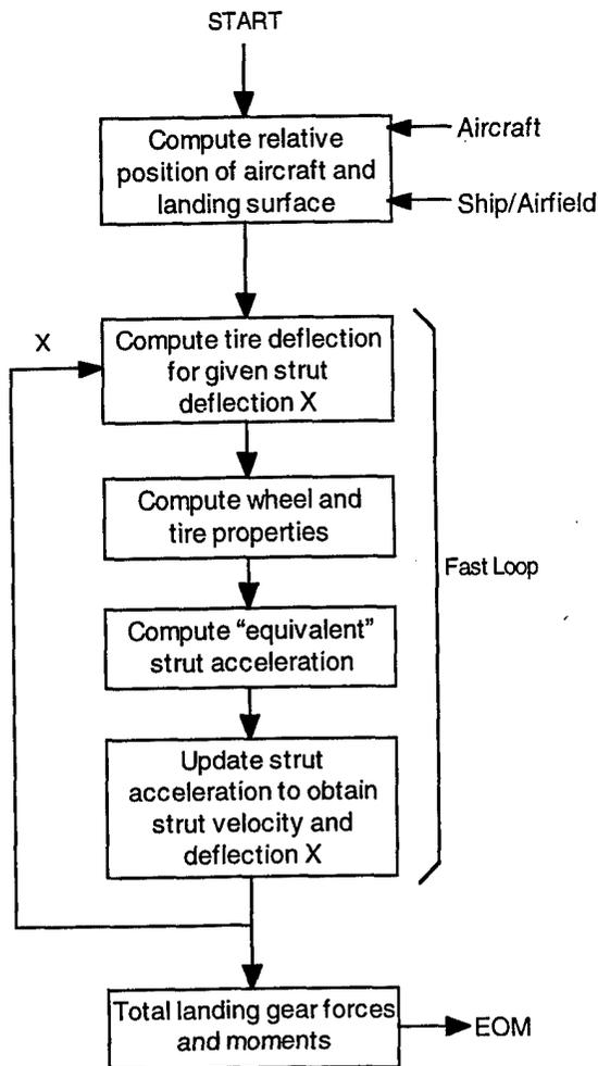
Figure 1. Landing gear model fast loop operation.
