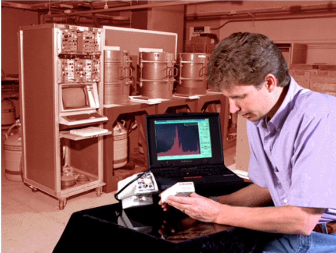
Figure 2. The portable radiation detector being demonstrated by its inventor Anthony Lavietes can identify the precise isotopic signature of nuclear materials such as plutonium and uranium by detecting gamma radiation. It improves upon the large germanium-based detectors shown in the background and has a variety of applications, among them assistance with defense against terrorism using weapons of mass destruction.
