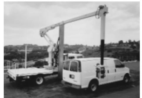
Figure 6. Mobile Gamma-Imaging System
