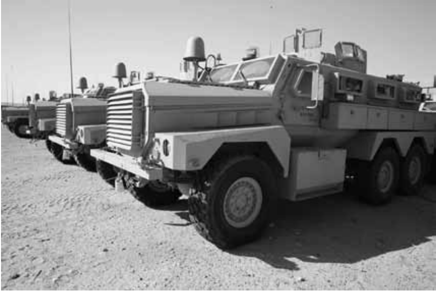
Figure 11.Ca Category II MRAP, used for convoy escort, troop transport, and explosive ordnance disposal
