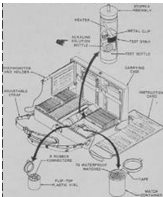
**Fig. 16-28.** The M272 Chemical Agent Water Testing Kit and its components. New kits have a test strip instead of a thermometer; this illustration shows both. Reprinted from Brletich NR, Waters MJ, Bowen GW, Tracy MF. *Worldwide Chemical Detection Equipment Handbook*. Edgewood, Md: Chemical Warfare/Chemical and Biological Defense Information Analysis Center; October 1995: 433. Drawing: Courtesy of US Army Edgewood Research, Development, and Engineering Center, Aberdeen Proving Ground, Md.
