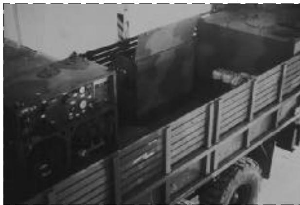
**Fig. 16-41.** The M12A1 Power-Driven Decontamination Apparatus (PDDA).
