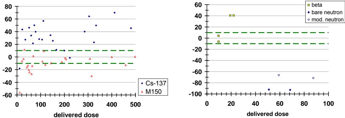
**Figure 4. ANSI N322 laboratory performance for SIRAD read by optical densitometer.** For each delivered dose on the x-axis, the percent difference of the optical densitometer result is plotted on the y-axis. Exact agreement between measured and delivered dose would be 0 percent difference. Points within the green dashed lines would meet the N322 accuracy test performance measure of 10 percent.
