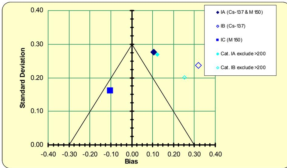
**Figure 5. ANSI N13.11 performance for SIRADs read by optical densitometer.** The bias (mean relative error) is plotted on the x-axis and the relative standard deviation is plotted on the y-axis for each category. Points within the triangle would pass the N13.11 performance criteria for the Accident categories.
