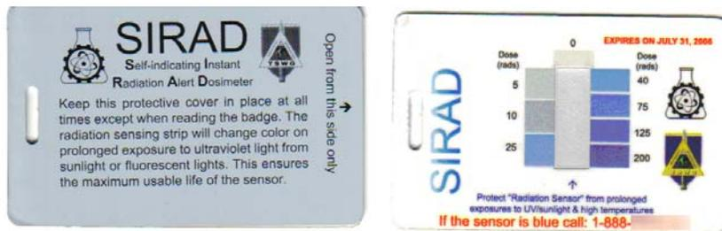
**Figure 1. Front of SIRAD card.** The image on the left shows a protective cover flap, and the one on the right shows the underlying SIRAD card with its radiation sensitive strip and color-matching scale. It was developed by Dr. Gordhan Patel, JPLabs ([www.jplabs.com](http://www.jplabs.com)) with support in 2003-2005 from the Technical Support Working Group (U.S. Departments of Homeland Security, Defense, Justice, and State). Its early development (1995-1997) was supported by the U.S. Navy.
