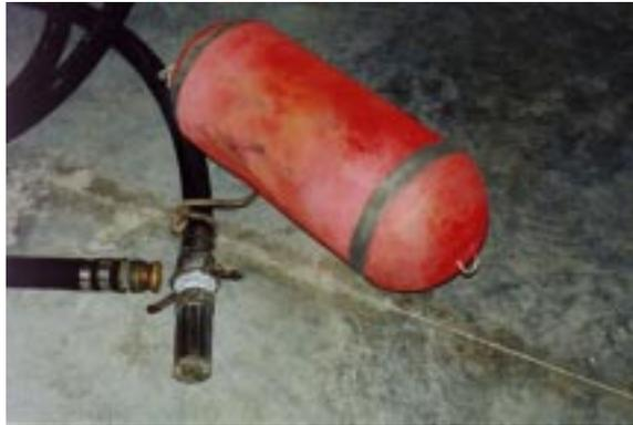
Suction Hoses (figure 15). Suction hoses are installed on the inlet side of most accessory pumps and are used to carry water to the pumps. They are hard walled, black in color, and have quick disconnect fittings. You will find both 1 ½” and 2” sizes in 10’ lengths. A few sections are marked with a blue stripe—the stripe denotes the hose should be used for product water only.
