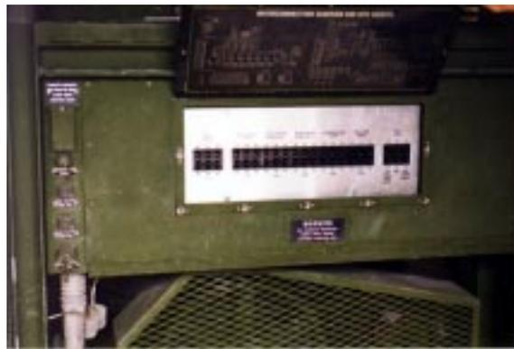
Control Panel (figure 4). The control panel contains the meters, valves and switches used to operate the unit. The panel also includes the coupling points used to connect hoses from various accessory components.
