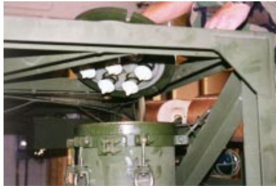
**Figure 44. Cartridge Filter Tube Replacement.**
