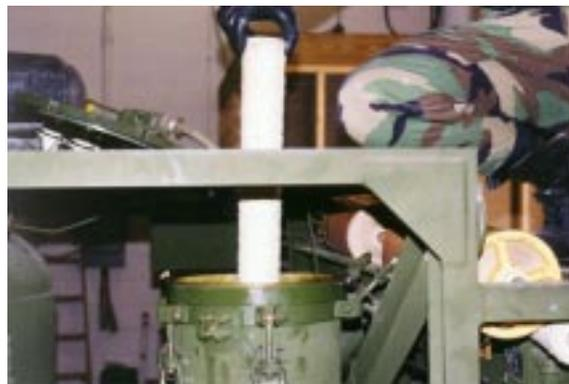
Rotate eyebolts into position and alternately hand tighten in the order shown in figure 45. Connect hose to the top coupling. Close access hole in canvas cover.
