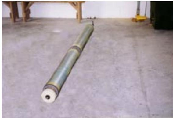
Clean the inside of the pressure tube with brine water. Also clean the end connectors and interconnector with a clean cloth. Check the end connectors, interconnector and all preformed packings (figure 50) for serviceability.
