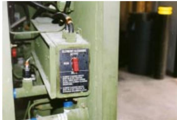
Loosen vent plug on top of backwash pump. When steady stream of water comes from around the plug, tighten the plug.
