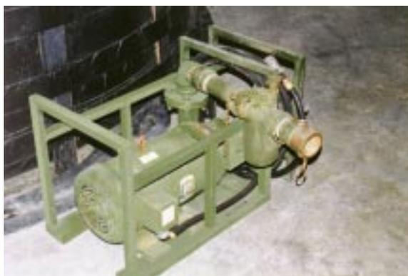
Install a 1 ½-inch female quick disconnect fitting on the 1 ½-inch gate valve.
