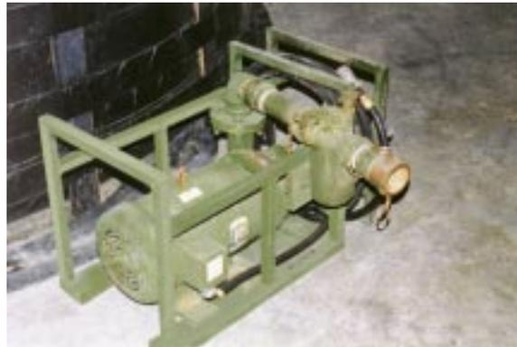
Raw Water Pumps (figure 13). Two of these electrically driven, 30 gpm pumps are used to draw raw water from the source and pump it to the ROWPU for processing.
