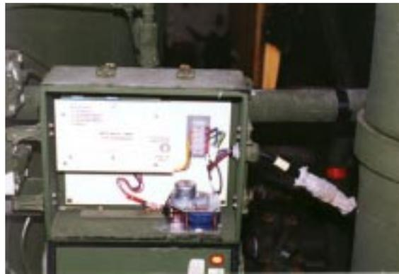
Once the initial unit preparatory actions are completed and the backwash valve is set to BACKWASH, the backwash timer comes on and controls the backwash process automatically. To backwash the multimedia filter take the following steps:
