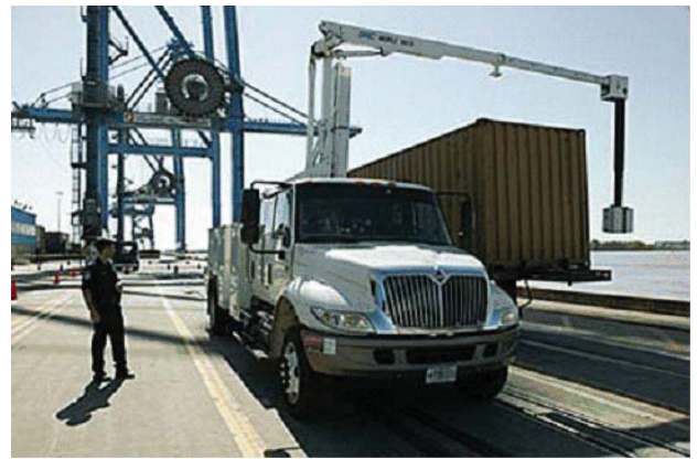
A seaport container is examined with a mobile truck x-ray
