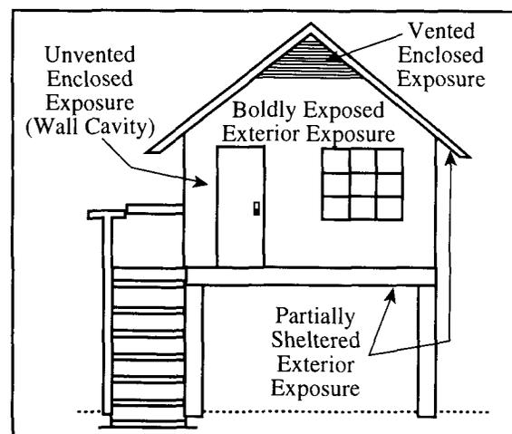
Figure 5. The locations of various classes of corrosion
