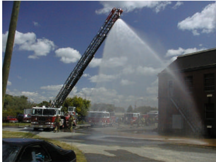
Figure 4-1. The Ladder Pipe Decontamination System
