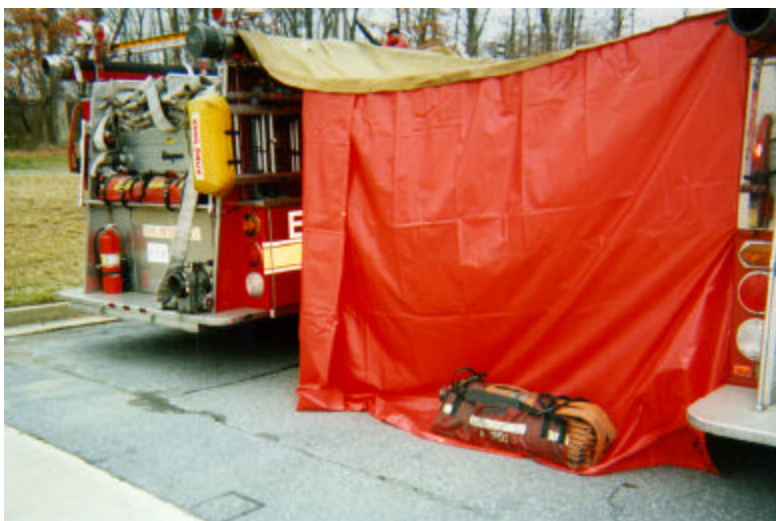
Figure 4-5. Proper Positioning of Salvage Covers Provides Adequate Privacy to Victims
