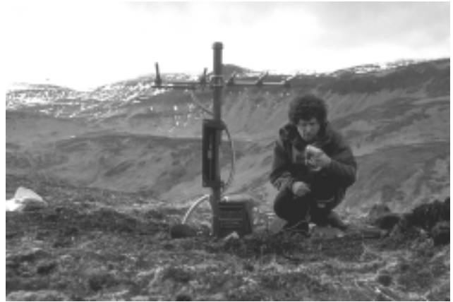
Figure 8. AVO seismologist John Power installing seismic station AK4, located on the south side of Akutan Harbor. Photo by R. McGimsey, 3/17/96.
