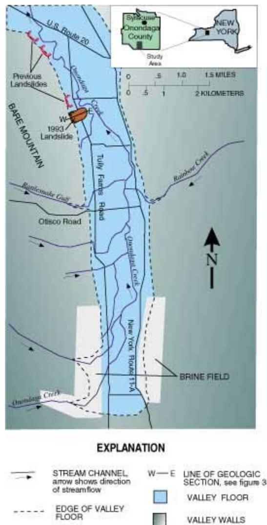
**Figure 2.** Major physical features in Tully Valley, including the 1993 landslide, previous landslides, and the brine-mining area at the southern end of the valley.
