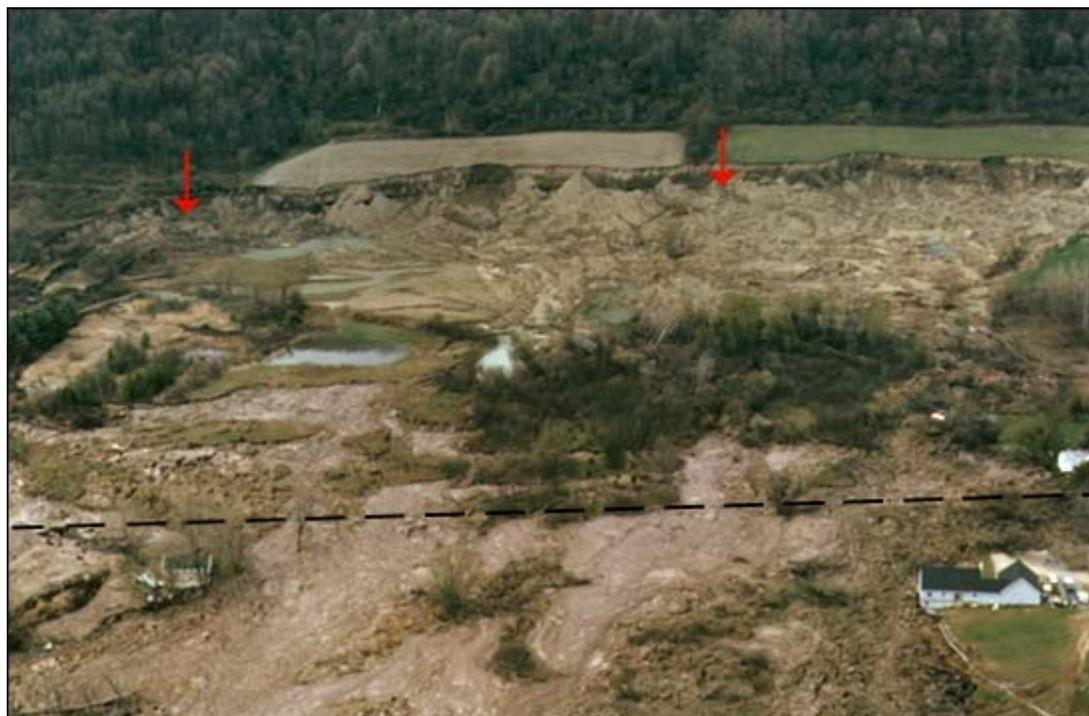
**Figure 1.** Oblique aerial view of the Tully Valley landslide taken April 30, 1993, 3 days after the slide. Debris moved toward the viewer, in the process covering Tully Farms Road (dashed line) up to 15 feet deep with reddish remolded clay. Three people were rescued by helicopter behind the white house (lower left) from the rapidly advancing landslide. Springs located between red arrows.
