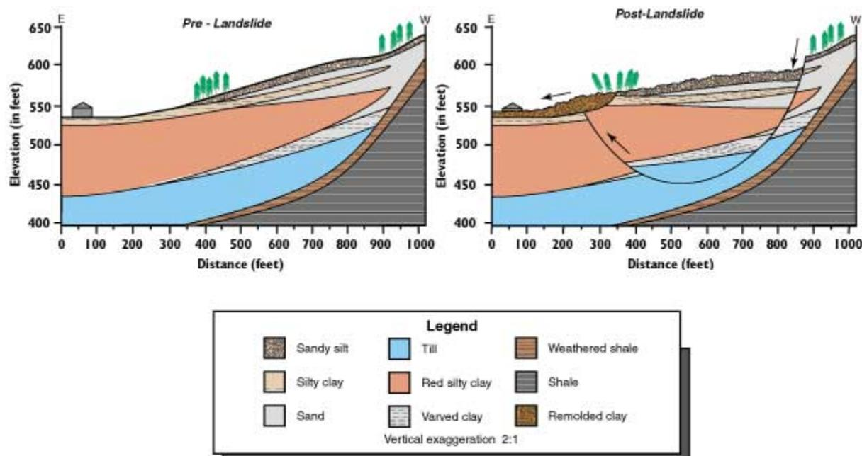
**Figure 3.** Soil stratigraphy before and after the 1993 landslide.
