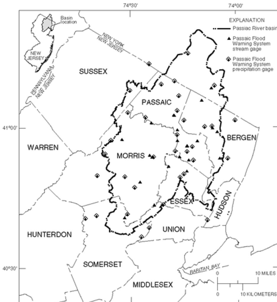
**Figure 1. Location of gages associated with the Passaic Flood Warning System in the Passaic River Basin and vicinity.**
