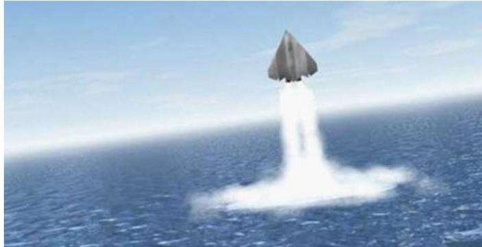
**Figure 22-Submarine-launched "Cormorant" UAV**
