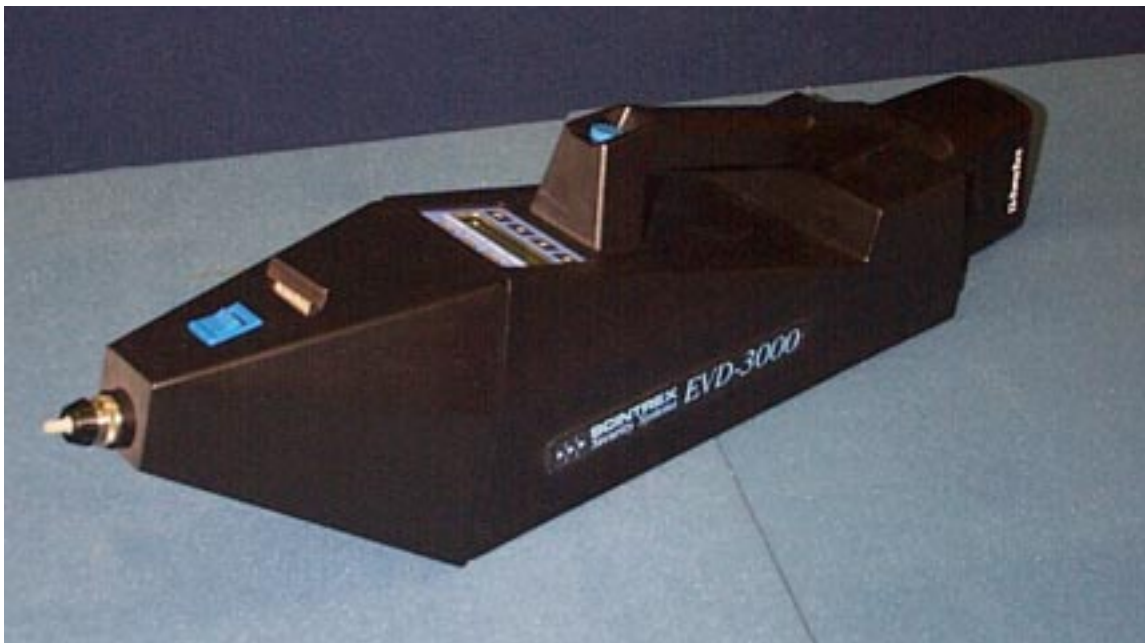
Figure 11. Photo of a Thermo-Redox detector, Sintrex/IDS EVD-3000
