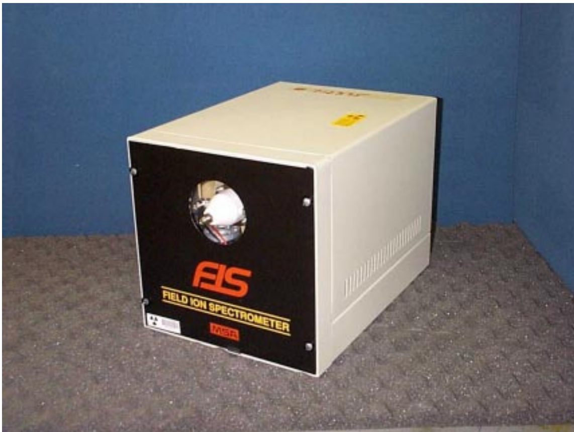
Figure 12. Photo of a field ion spectrometer (FIS) by MSA
