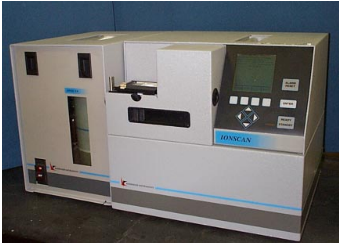
Figure 4. Commercial IMS explosives detection system, Barringer Ionscan 400
