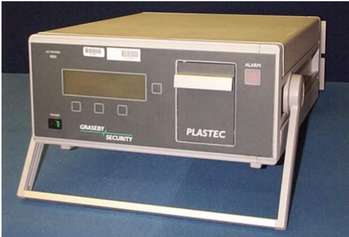
Figure 5. Commercial IMS explosives detection system, Graseby Plastec
