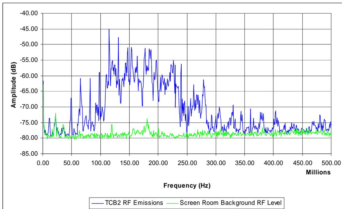
Figure 17: RF Emissions from 20 MHz to 400 MHz
