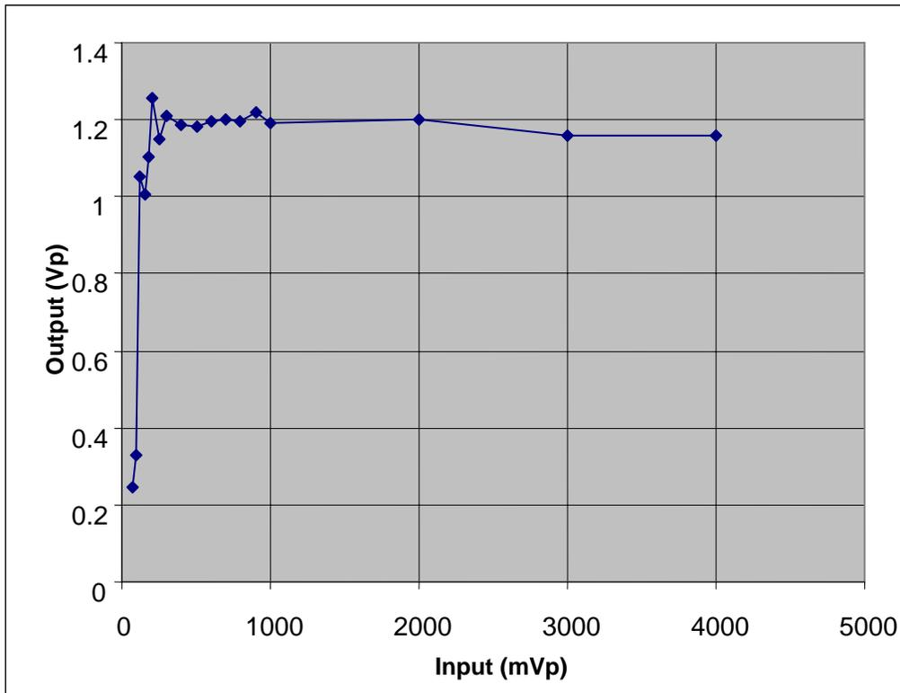
Figure 7: Audio Output Level Versus Input Level with AGC on at 50 Percent TX Level
