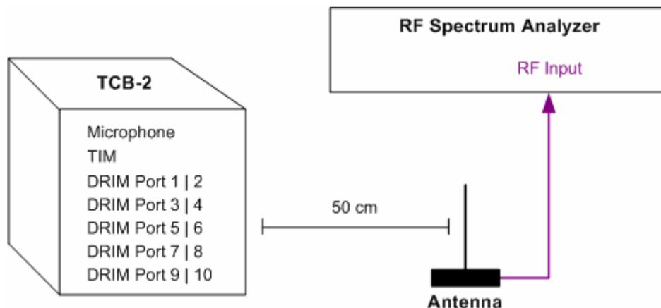
Figure 16: RF Emission Measurement
