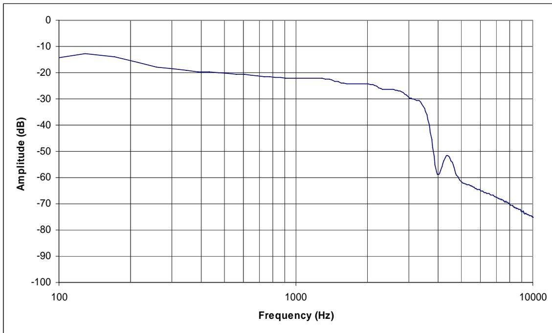
Figure 10: Frequency Response Input (Microphone), Output (Port 7).
