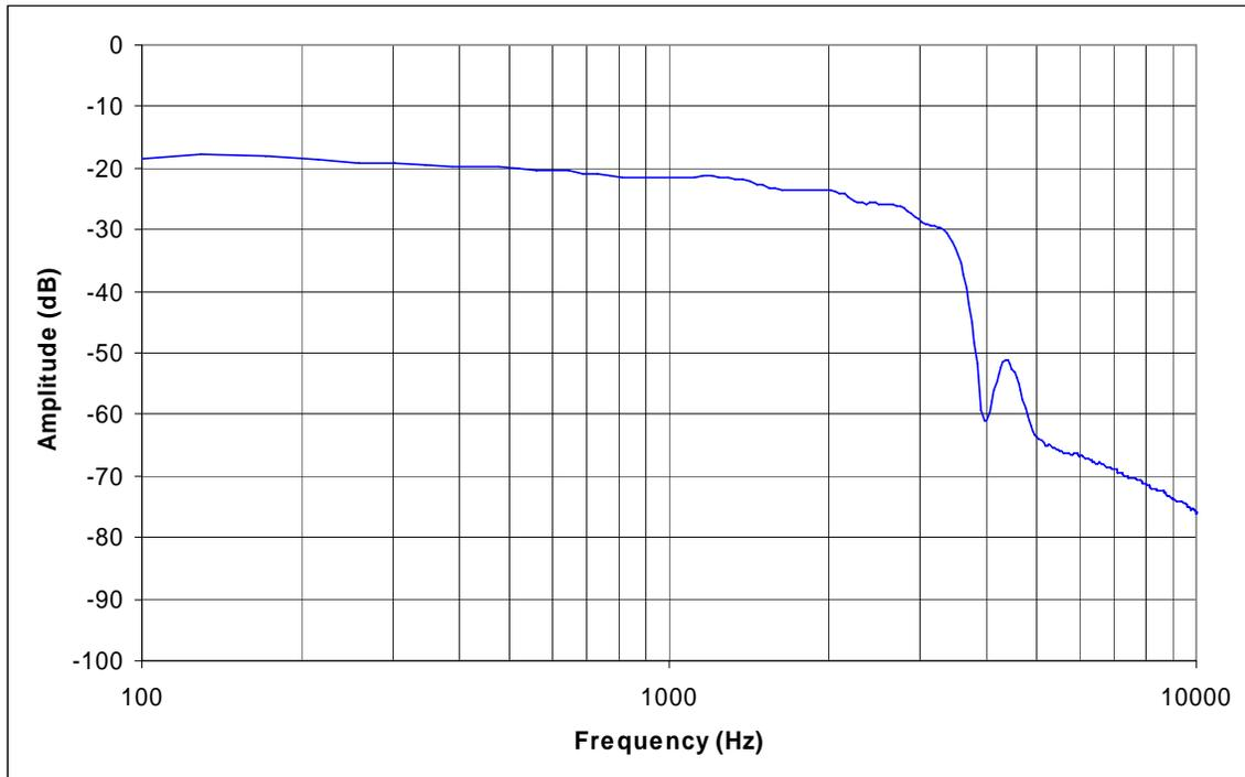
Figure 9: Frequency Response Input Port 3 to Output Port 7
