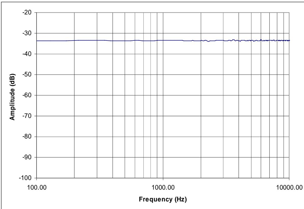
Figure 11: FFT of Input Noise Used to Determine Frequency Response
