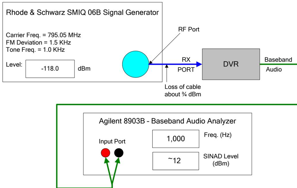
Figure 8: Block Diagram of Receiver Sensitivity Test
