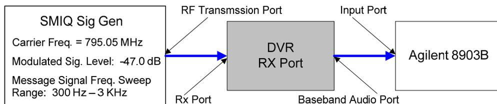
Figure 11: Block Diagram of Receiver Frequency Response Test
