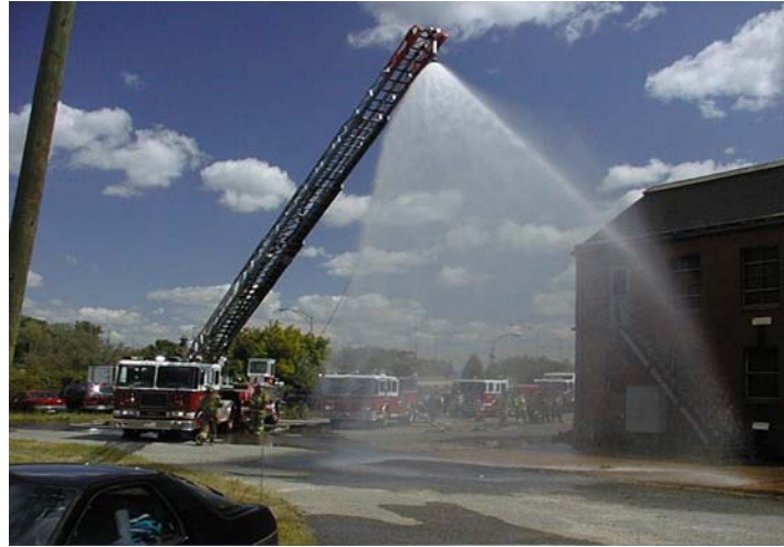
Figure 4-3. The Ladder Pipe Decontamination System (LDS)
