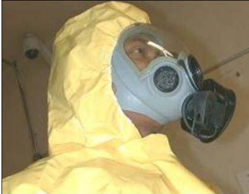
**Figure 6. Neck Leakage Around Suit Hood When Suit and Respirator are Worn Without a Respirator Hood**
