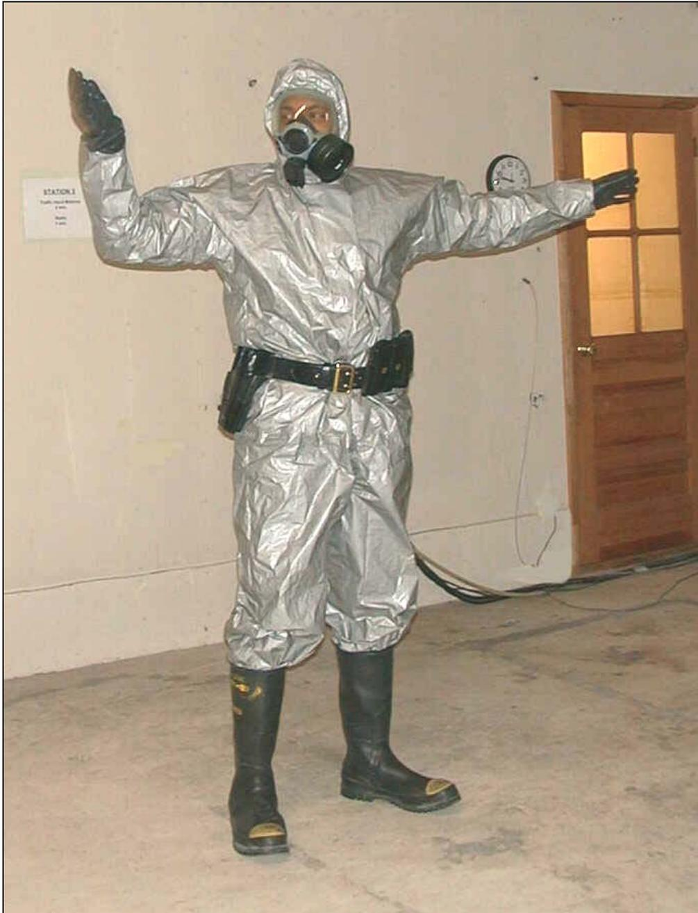
**Figure 5. Tyvek ® F Suit with Worn with Respirator, Respirator Hood, and Suit Hood (Double Hooded)**
