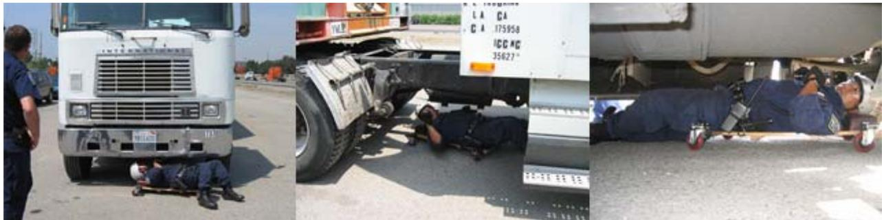
Figure 3: Truck Underbody Inspection
