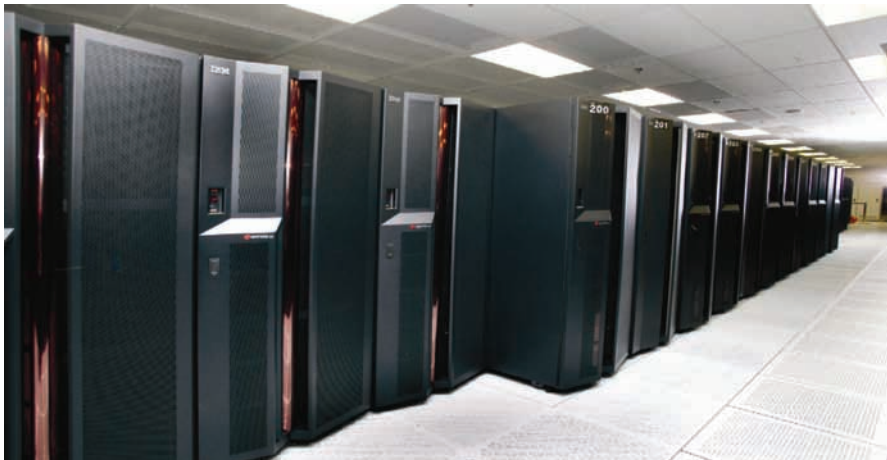
ASC PURPLE: One section of ASC Purple, which is capable of achieving a speed of 100 teraflops.
