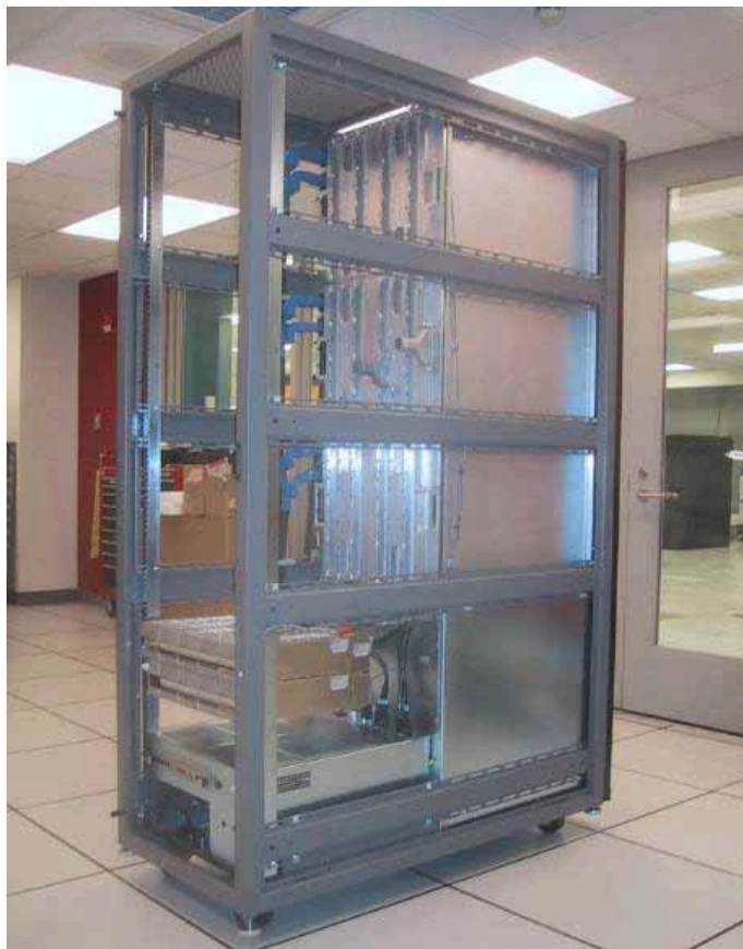
CALM BEFORE THE STORM: Red Storm, an air-cooled supercomputer, is being developed by Sandia and Cray Inc. using mostly off-the-shelf parts. A unit is pictured here in its initial stage of construction.
