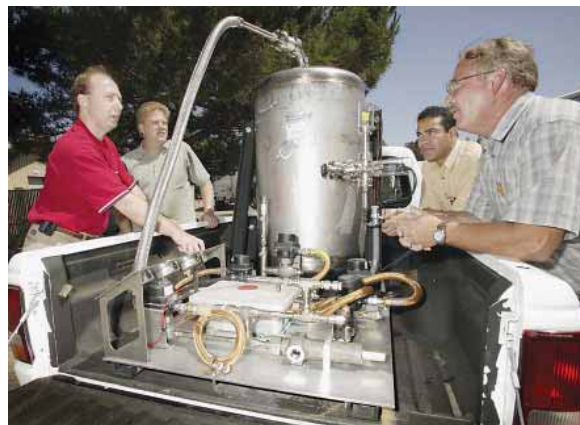
HYDROGEN FUEL RESEARCH: LLNL researchers (from left) Mark McCuller, Jim Fugina, Francisco Espinosa-Loza and Tim Ross discuss the LLNL insulated hydrogen fuel storage system installed in the back of a hydrogen-powered pickup truck.
