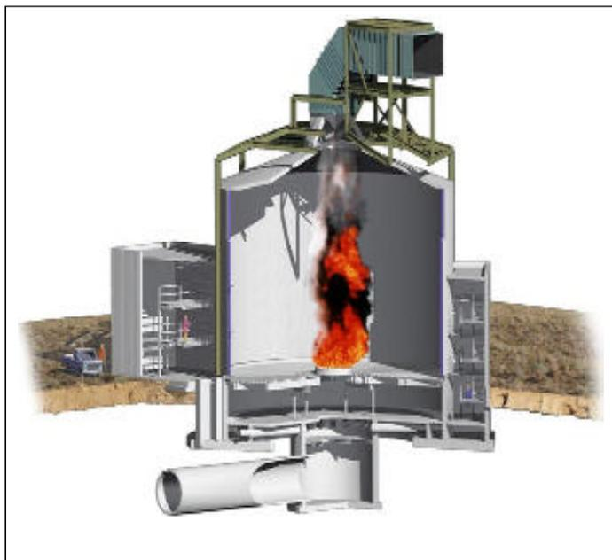
**THERMAL TEST COMPLEX:** Architectural drawing of 7-story FLAME Test Cell at the Thermal Test Complex, now under
